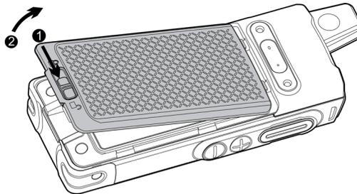
3. Lift the bottom of the battery to remove the battery from the radio.
