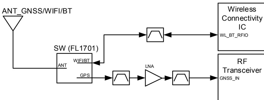
The GNSS signal goes to the Switch through the GNSS/WLAN/BT three-in-one antenna, and then it is shunted to the pre-filter for LNA amplification. Afterwards, the amplified signal passes through the
