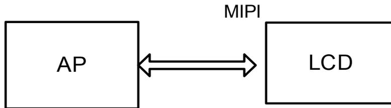
AP is connected to LCD (a 2.0-inch screen with resolution of 320 x 240) through MIPI.
