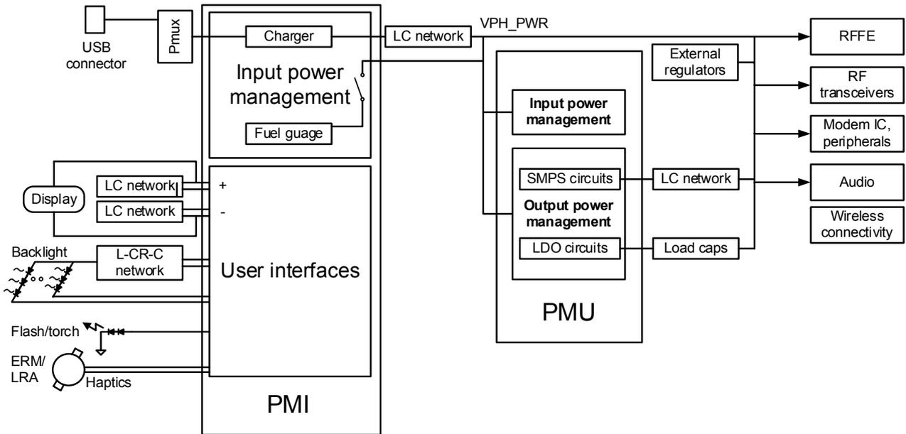
The power supply employs a 3.7 V battery. The power supply management IC consists of PMI and PMU.
