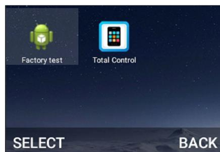
3. Select **Factory test**. (If **Factory test** does not appear on the interface, run the **open test** file to make it show up. If the screen turns to black and white when power-on, the terminal enters the FFBM mode.)
