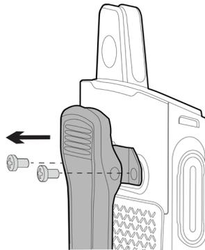
2. Slide the battery latch to the
